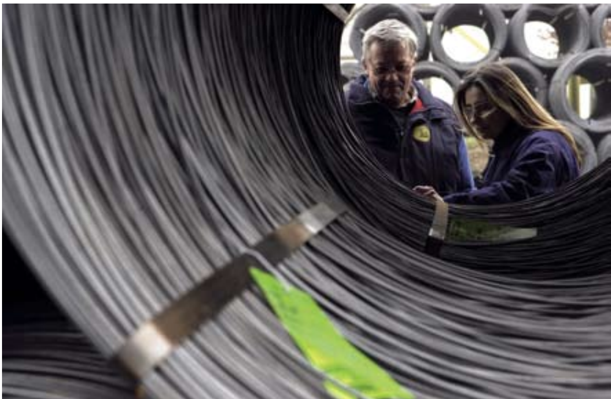
Wire rod is Bekaert's most important raw material. Bekaert buys wire rod in many different qualities and compositions to meet the most diverse production specifications.
